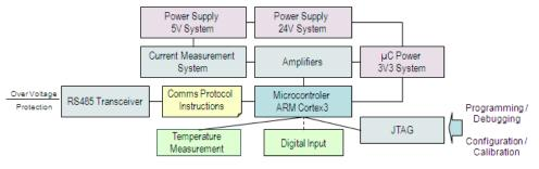
Figure 2: CMC SNV018EC Functional Diagram.
