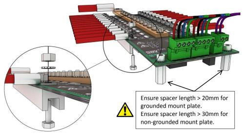
Figure 13: Detail view of "bolt holding bar" mounting
