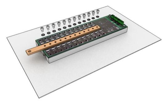
Figure 8: Mounting the common bar on the CMC SNV018EC
