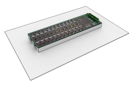
Figure 7: Placing the card on the mounting bars
