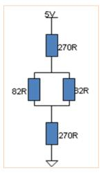
Figure 15: Bus termination and Bias resistors
