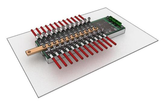
Figure 9: Mounting of the current measurement cables
