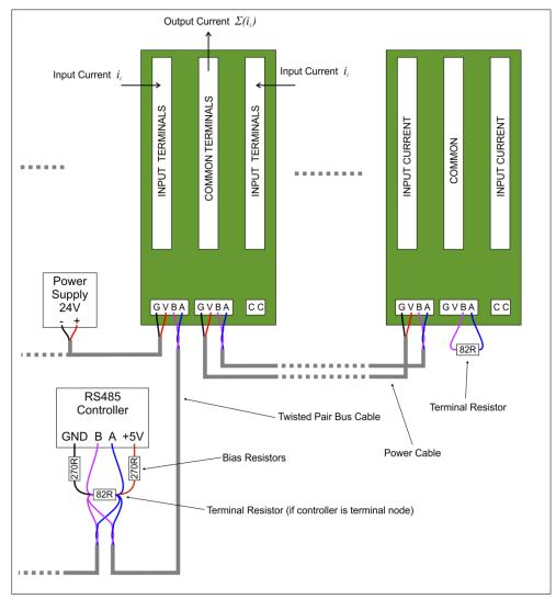
Figure 14: General Bus connection diagram.
