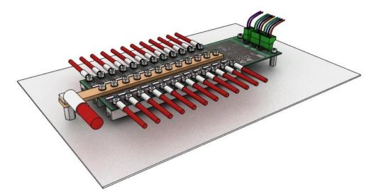
Figure 12: Alternative mounting figure with "bolt holding bars"
