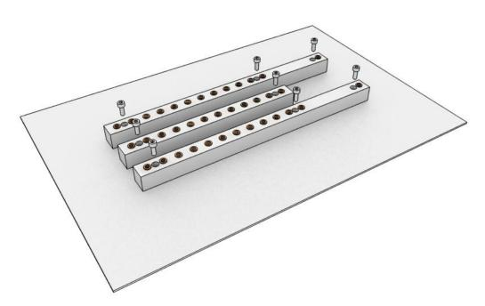
Figure 6: Mounting of the fixing bars
