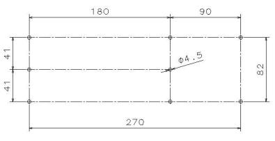
Figure 5: Drilling pattern
