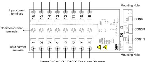
Figure 3: CMC SNV018EC Topology Diagram.
